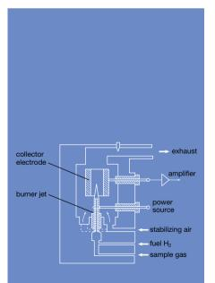
Employs the hydrogen flame ionization detection method featuring superb response characteristics and stabilitiy. Allows highly sensitive and highly precise continuous measurement.
