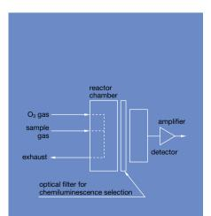
A nitrogen oxides analyzer based on the atmospheric pressure chemiluminescence method.
